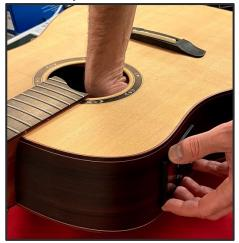
• Insert the HyVibe System in the preamp hole and connect the wires with your hand inside the guitar. After being properly plugged, the wires will look like the picture below:
