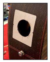
• Remove protection label, insert output/input/USB jack, and screw the housing into the guitar using the four 2x7 screws.
