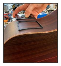
Mark 4 drill spots: place the HyVibe blueprint in the chosen location, and then indent tiny holes into the wood at each of the four corners of the inner rectangle on the HyVibe blueprint.
