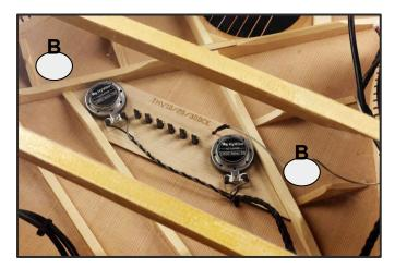
• Make sure the surface of the wood is clean, apply glue to the actuators and push them against the wood for ~10 seconds to confirm they are attached strongly. Make sure that they are arranged so the connector cable is directed to where the HyVibe System will be inserted.
